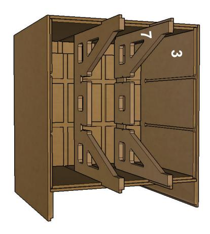
Important: The "brace tips" should be flush with the LEDGE on Panels 1 and 5. Do not force them in any further than the ledge itself. Try to position them to be exact!
