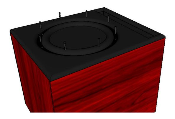
Using the 7/64" drill bit, drill the 8 driver mounting holes. The supplementary driver mounting ring provides two layers of MDF for the screws to attach to. This provides maximum holding power and minimizes the chances of stripping even one screw.
