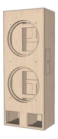
Start: Driver mounting rings. The rings with the smaller diameter are mounted on top of the assembly.
