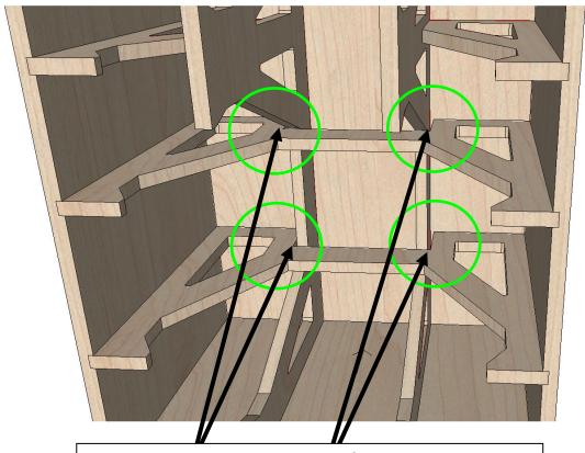
There is a 0.25" gap between the full-width horizontal brace cutout and the vertical braces. DO NOT ATTEMPT TO CLAMP THESE PIECES TOGETHER.
