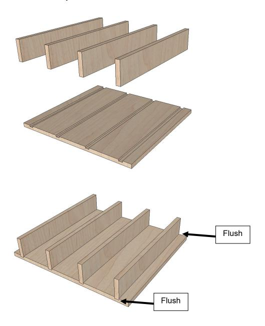
Attach rear port board and bottom port board to side panel.
