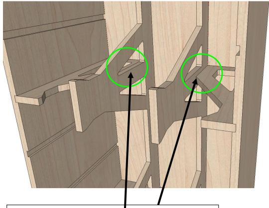
Where the small braces contact that vertical brace, be sure to apply glue and clamp them together.
