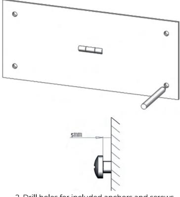
2. Drill holes for included anchors and screws.
