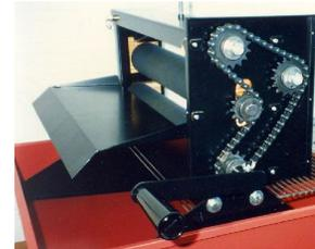
Heavy duty roller chain positive drive ensures both roller drives thorough travel
