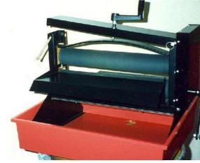
EXTRACTOR Quick release pin and Adjustable leaf spring
