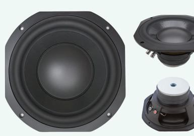
The SB2550 uses a heavy, doped cone, large rubber surround and a rigid plastic dustcap that can make high excursions with true piston movement. The stacked magnet assembly is rear vented for cooling and is deep enough to allow exceptional peak to peak travel well in excess of the substantial linear capability without bottoming out.
