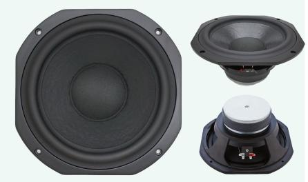
The B251.8 features a symmetrical field magnet and long voice coil for large linear excursion capability. It also has double rear suspensions whose characteristics are matched to that of the motor assembly for stability and linearity at high drive levels. An extended centre pole is utilised to minimise distortion inducing inductance swing at high power levels. The Thiele-Small parameters are optimised for bass extension.
