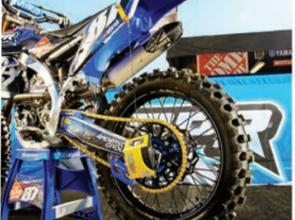
Draw out the retractable cable and hook it to the clamp or hole that you drilled. Power on Slacker using the power button to the left of either display. Make sure Slacker is angled along with the cable.
