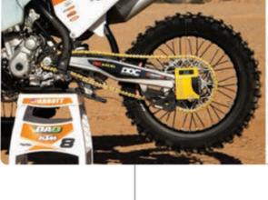
**!** For 2016 and newer KTM and Husqvarna bikes measure to the sag mark on the rear fender. This will be more vertical than the arc method above. You can also drill a small hole in the lip of the plate or fender to speed up the process.
