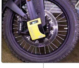
Draw Slacker cable out, hook it to the adapter, and turn it on using the power button on the left side of the display. The retractable cable should line up with the forks and be perpendicular to the top edge of Slacker.
