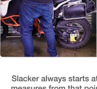
Place Slacker in Auto Zero mode by holding down the backlight button on the right side of either display. Once the cursor begins to scroll, lift the bike to top out the shock. Slacker will automatically find the zero point and you can now start taking measurements in real-time.
