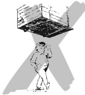
After lifting or tensioning, a load must not be left unattended or remain lifted for a longer period of time.
