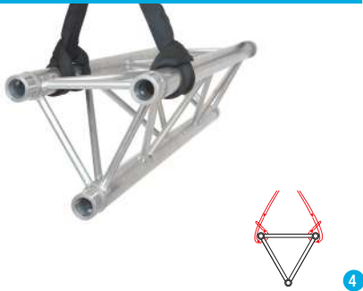
TRIANGULAR TRUSS | APEX DOWN 2 SLINGS, CHOKES ON TOP CHORDS
