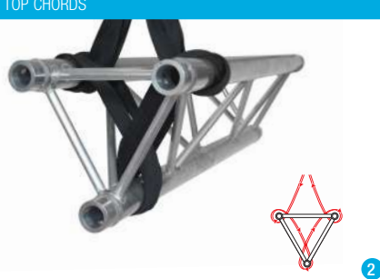
TRIANGULAR TRUSS | APEX DOWN 1 SLING, BASKET ON BOTTOM CHORD AND WRAPS ON TOP CHORDS
