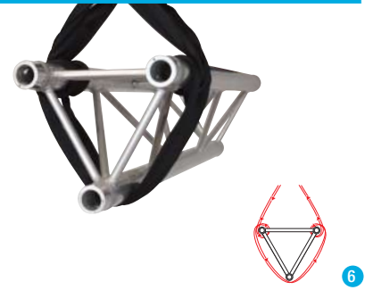
TRIANGULAR TRUSS | APEX DOWN 1 SLING, BASKET WITH WRAPS ON TOP CHORDS
