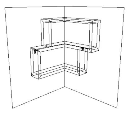
4) Use a pencil and make a mark on the wall in the center of the lower hole of the L-bracket.
