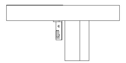
3) Hold the shelf in position approximately 2" higher than where you actually want the shelf to be located. (There may be a small gap between the shelf and the wall. This is ok and will not affect the stability of the shelf.)
