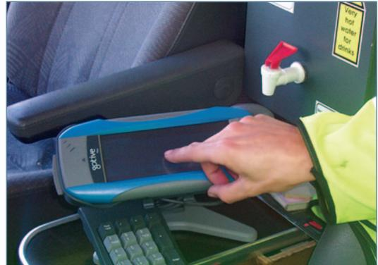
about the type and state of repair of the unit and whether a revisit is required to attend specific faults. The information is paired with Coordinates from the in-vehicle GPS system and automatically sent (using GPRS) to RCS's central database in Basingstoke.
