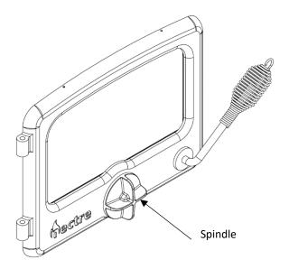
A tool for opening and closing the spindle is supplied with the heater. This can be used in instances when the spindle control is too hot to touch. Alternatively, a glove or equivalent can be used to adjust the spindle.
