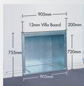
Zero Clearance Box positioned in framework mounted on 12mm Villa Board cut out size. (Box size: 905w x 720h) (Cut out size: 905w x 755h)
