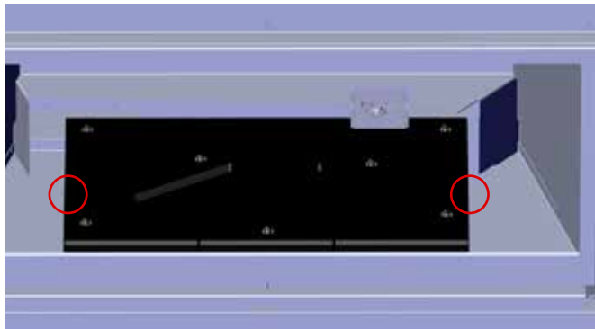
Diagram 2 - Burner Screw Locations
