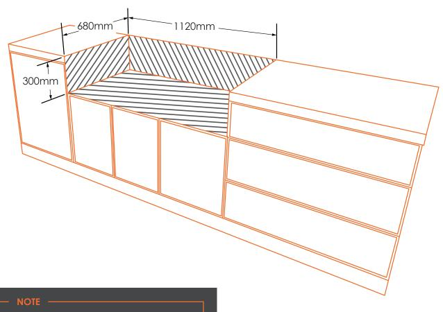
Minimum clearance to combustible wall surfaces above the BBQ body cooking surface is as follows:
