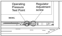
Check the inlet pressure to the appliance. Attach manometer tube to the first test point upstream of the appliance (typically at the gas utility meter or auto change device for a propane bottle station)
