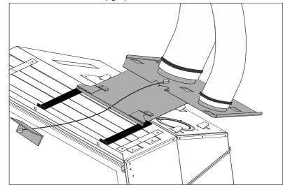
Make sure that all six of the fold up tabs (shaded in the diagram below) used for locating the flue spigot plate onto the chassis are poking through the flue spigot plate.
