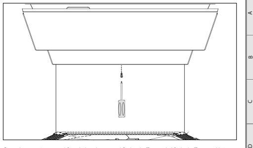
Once the screw is removed from below the stepped firebox baffle, gently lift the baffle up and bring towards you. Remove the 8 machine screws in the access panel (as shown in the diagram below).
