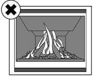
An abnormal flame pattern will likely be the result of incorrect settings (jet size, burner aeration collar, flue restriction), and if present you must check these are correct before proceeding. If an abnormal flame pattern is still present, please contact Escea.
