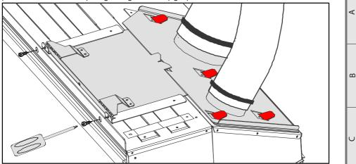
Insert the 2 long self tapping screws into the location shown in the diagram above to secure the flue spigot plate to the chassis.
