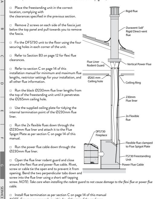
□ Install flue termination as per section C on page 14 of this manual NOTE: Ensure a power supply is within 1m of the rear of the appliance.
