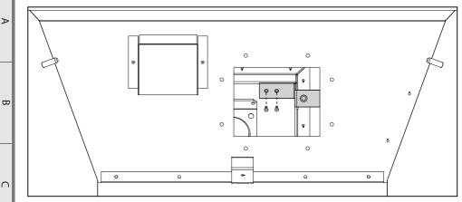
Disconnect the two wires from the TCO and the bracket with the TCO may then be removed from the fire box for replacement.
