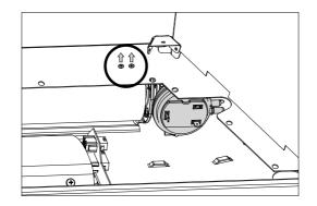
The bracket with the pressure switch may now be removed from the firebox.
