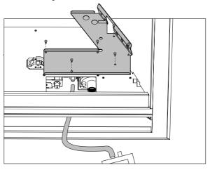
Adjust the operating pressure by feeding a screw driver through the front face of the fireplace and turning the regulator adjustment screw.
