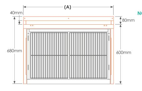
**NOTE** When Roasting hood is shut, handle will pass front panel by 32.2mm this makes the hood to be 576mm deep.
