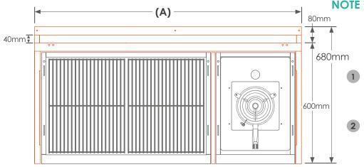
When Roasting hood is shut, handle will pass front panel by 32.2mm this makes the hood to be 576mm deep.
