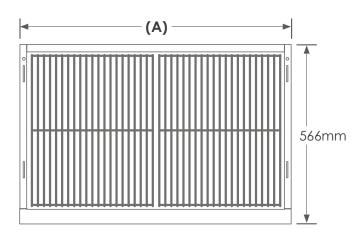
NOTE When Roasting hood is shut, handle will pass front panel by 32.2mm this makes the hood to be 576mm deep.
