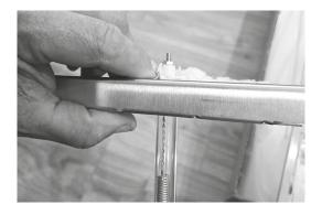
The element, end with the wider end panel placed over it, locates into a hole at the opposite end to the junction box.
