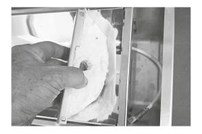
4. Now, carefully pick up the glass element and remove 1 x press nut and washer from each end and then slide one end panel over each end of the element then lay the element back down into the heater.
