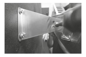
Both the triangular and the U shaped mounting brackets have 4 attachment holes in one end of them which when used to attach the 2 x mounting brackets together, can secure the heater at either 45 degrees from a ceiling or wall or secure it at 90 degrees from a ceiling or wall.
