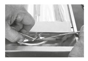
**NOTE <u>Do not</u>** try to turn the fixed press nut, only turn the outside nut.
