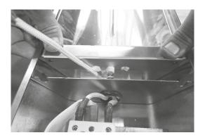
7. Place the wire lug found at each end of the heater onto the ends of the element, then place a standard washer (supplied inside the bag of fixings), spring washer and press nut back onto each end of the element to hold the lugs on the element.
