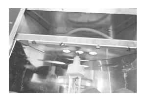
Then carefully locate the other end of the element, that has the narrower end panel sitting over it, into its position in the half round cut out at the opposite end of the heater.
