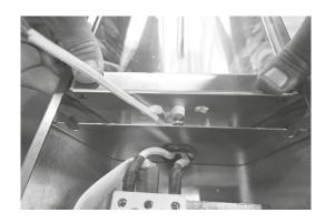
7. Place the wire lug at each end of the heater onto the ends of the element, then place a standard washer (supplied inside the bag of fixings), a spring washer and then a press nut to secure them onto the element at each end.
