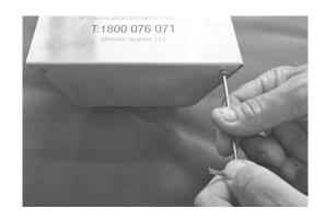
NOTE Always check to ensure that the rubber sealing pad is correctly positioned around the nylon gland before tightening.
