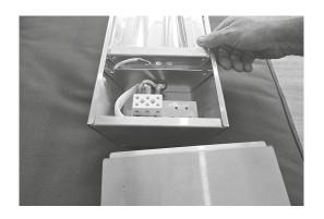
2. Remove the safety grill from the heater by pulling out the spokes from underneath the lip on one of the long sides of the heater first and then removing the spokes from the other side next, then gently lift the grill up from its center while carefully removing the grills spokes from the end panels, one end at a time.
