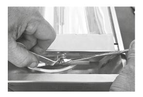
**NOTE** <u>Do not</u> try to turn the fixed press nut, only turn the outside nut.
