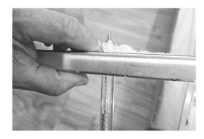
5. Slide the end of the element, that has the wider end panel placed over it into the locating hole at the opposite end to the junction box.
