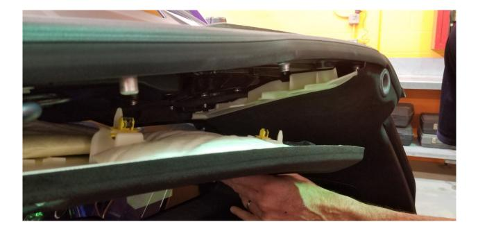
6. To loosen the rear driver closeout panel behind the driver's seat, use a plastic prybar between the panel and the body of the car inside of the door jamb. Gently pop the panel out to release three clips, which will allow the panel to be moved out far enough to access the X900 connector.
