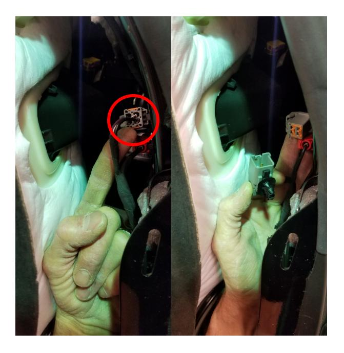
Plug adapter into the corresponding male and female ends <u>without bending the middle of</u> <u>the Adapter</u>. Push the rear of the connector towards the back of the car and place it between the seatbelt retractor and the inside body. The ends of adapter may be bent slightly to allow it to fit under the rear panel.
