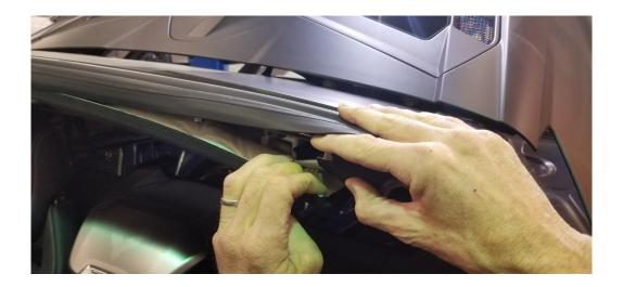
4. Using a panel popper (or screwdriver), carefully pull down the headliner and release the four front clips.
