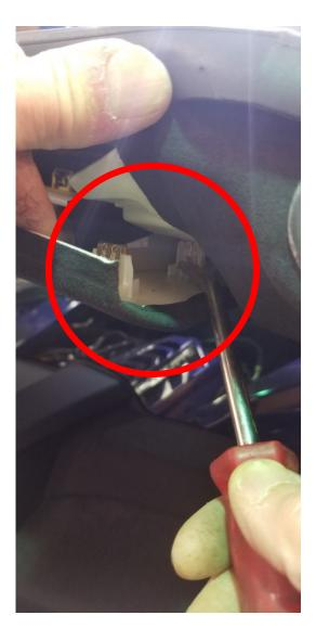
5. Using a long screwdriver or panel popper, release the two remaining clips that are on the very edge of the headliner of the driver's side. The entire driver's side of the headliner should now pull down about six inches.
