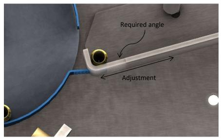
INSTALL THE TORCH IN THE HOLDER. NOTE THAT THE TANK ITSELF IS PROBABLY AS HEAVY AS YOUR ECHO ANNEALER, SO POSITION IT SO THAT THE TORCH BASE IS RESTING ON THE TABLE IN A WAY THAT THE MACHINE REMAINS STABLE, AND THE TORCH POINTED TOWARDS THE NECK PORTION OF THE BRASS.
