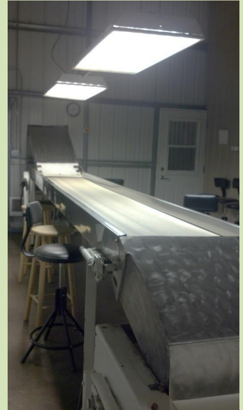
Larger volume nut sorting conveyor
