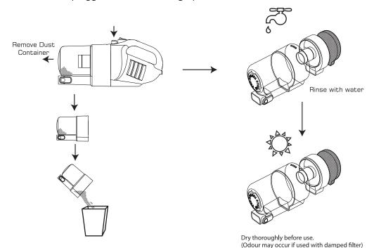
Cleaning tools can be wiped and cleaned by wet cloth but no immersing in water as it may cause damage. Cleaning tools must be completely dry before putting into operation.
