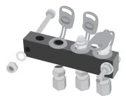
Screw the threaded sleeve (A) onto the hose (D) (sleeve is reverse, or counterclockwise, threaded) until the threaded sleeve is bottomed out on hose.
