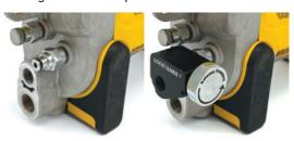
6. Fit the Banjo bolt through the valve body and into the grease hose port ensuring that the dowty washers are in place above and below the valve body. Do not over tighten the bolt.
