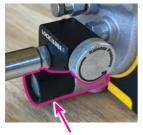
8. Ensure that the thumb screw is hand tight (turn clockwise to tighten)
