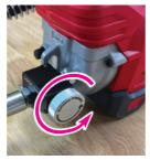
When the pressure in the grease hose needs to be released, unscrew the thumb screw a single turn. This will allow grease to flow back into the barrel.
