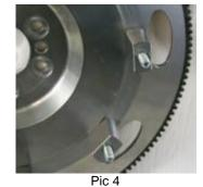
6. Mount the clutch disc with the part number suffix "-F/X" onto the flywheel with the side marked "Flywheel Side" against the flywheel and insert an alignment tool through the clutch disc spline.
