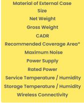
ABS 284 X 173 X 439mm 3.4kg 5.5kg 208m<sup>3</sup>/h Up to 21m<sup>2</sup> 53dB AC 220-240V, 50Hz 0 to 40°C / 20 to 90% No Dew -10 to 60°C / 20 to 90% No Dew Wi-Fi IEEE 802.11 b/g/n 2.4GHz
