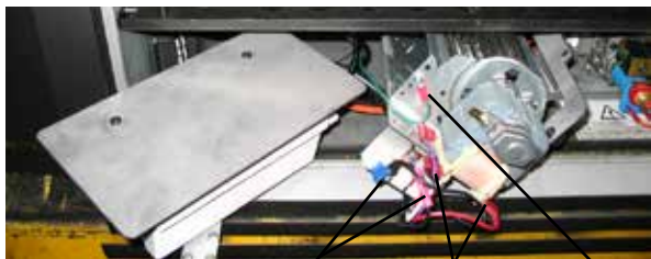
Resistor Connectors Fan Connectors Fan Ground Cable
