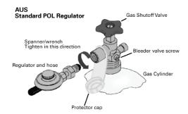
To turn the barbecue 'OFF', turn the cylinder valve to the 'OFF' position and then turn all of the control knobs on the appliance clockwise to the 'OFF' position.
