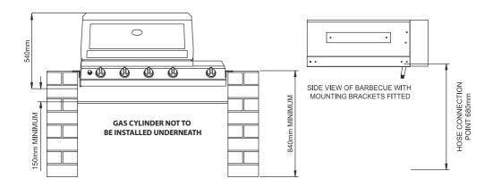
NOTE: TO BE INSTALLED BY AN AUTHORISED PERSON. PLEASE NOTE: MINIMUM CLEARANCE TO COMBUSTIBLES UNDER FAT TRAY IS 150mm. THE MATERIAL FOR THE CABINET (ISLAND) MUST NOT BE COMBUSTIBLE.
