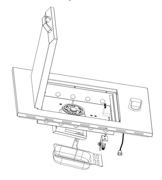
3. Remove the connector (With LPG & NG injector)
