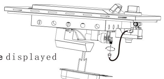
4. Remove the LPG injector, the NG injector will be displayed
