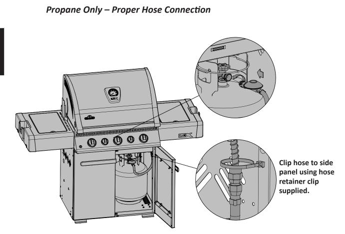
Ensure the regulator drops into the small opening, between the tank heat shield and the right side of the cabinet.
