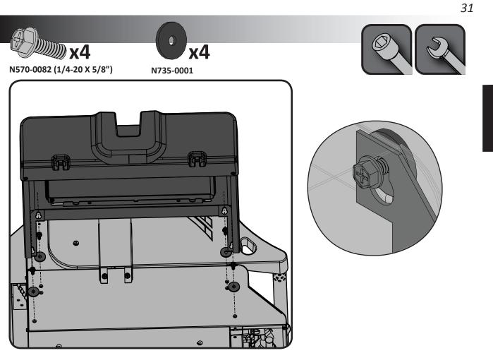
Tabs located on either side of ice bucket must engage notches in side shelf.
