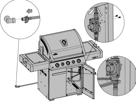
This unit includes an internal regulator which stabilizes the gas pressure and improves grill performance. This regulator cannot be adjusted. There is a pressure tap located on the side of the regulator. It can be used by a qualified service person when servicing the grill to determine if the regulator is functioning properly. The screw within the pressure tap must always be kept tight, except when performing a pressure test on the regulator (qualified service personnel only).
