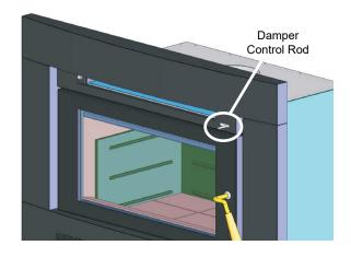
6) Install knob on damper control rod.
