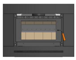
5) Install the draft plate cover by sliding the tabs into the tab brackets on the inside top of the firebox, ensure the damper control rod fits thru the opening in the draft plate cover.
