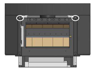
**3)** Install the fan fascia by aligning the bottom screw locations with the bottom faceplate. See page 13 for fan wiring diagram.
