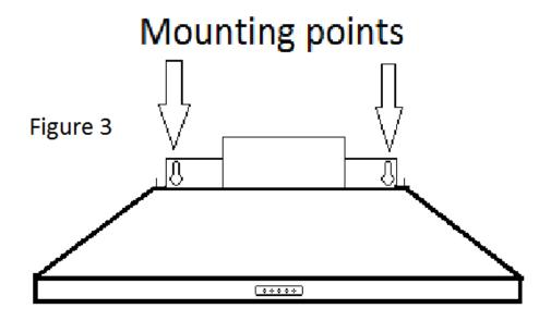
Step 5: Screw fixings into marks for mounting
