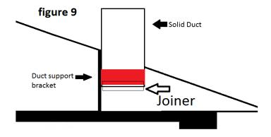
Connect one end of the flexible duct to the stating pop on the rangehood. Secure this with some PVC duct tape. See figure 9
