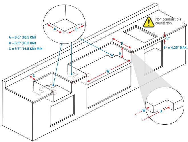
**E**\*= For use with the installation of a Napoleon BI door.
