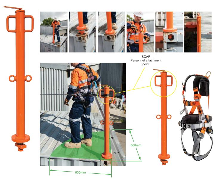
Before using the SCAP, the user needs to be equipped with appropriate PPE and a full body harness compliant to AS/NZS1891.1. An SRL shall be attached to the SCAP personnel attachment point which gets attached to the harness of the user.
