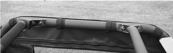
2. The rear edge of the doors has 3 strips of Velcro sewn down the entire length. Starting at the top use the 6", 16" and 8" adhesive strips to attach the door to the roll cage. This attaches to the Velcro sewn down the sides of the rear window. See photos below.
