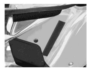
5. Finally, the bottom of the door has three snaps, one on the inside and two on the outside. Best way to put the screw studs in the correct place is to install the screw stud into the snap on the door first. Then pull the door in place and push the point of the screw into
