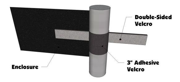
3. The diagrams below show how the double-sided straps and the 3" adhesive Velcro works.
