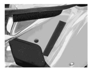
5. Finally, the bottom of the door has three snaps, one on the inside and two on the outside. Best way to put the screw studs in the correct place is to install the screw stud into the snap on the door first. Then pull the door in place and push the point of the screw into the plastic making sure to leave a good mark. Then pull the snap stud out of the door and screw into the plastic where the mark was left. See photo below.
