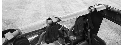
7. The sides of the Rear Window will attach to the Velcro tabs from the doors. The one exception is the top corners that have a double-sided tab that is held in place by a 3" adhesive strip. The bottom of the Rear Window will hang between the bed and the backs of the seats. See photos below.
