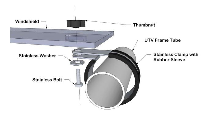
**8.** Next place the top windshield section on the roll cage. It should mate with the bottom section as shown in the next few images.
