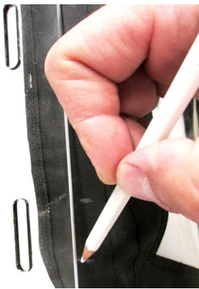
3. Mark the fabric where the slots are located. IMPORTANT: Carefully verify the windshield is positioned correctly!
