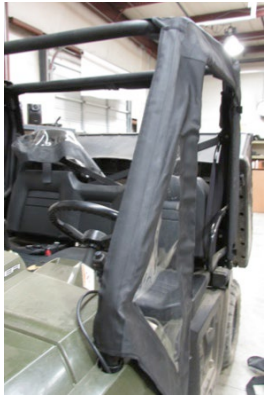
1. Mount side panel cab sections positioned correctly & taugth. NOTE: You will cut the side panels - Ensure they are positioned correctly.
