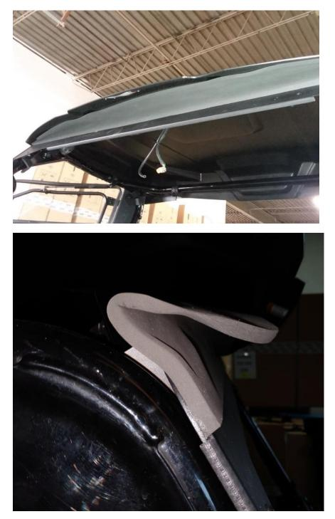
Tuck the rubber seal with your fingers into the underside of the roof and then bolt the roof in place.
