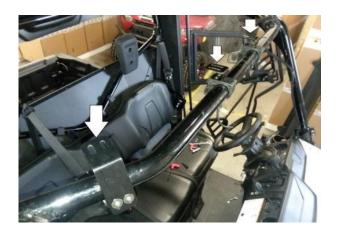
Install the 6 roof clamps on the ROPS (arrows above), positioning them below the predrilled holes so the roof is ready to be bolted down. Screw in the back 2 brackets so the roof will lift up and down in the front without losing position.
