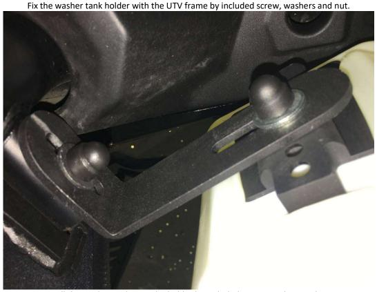
Install the washer tank onto the holder by included screw, washers and nut.
