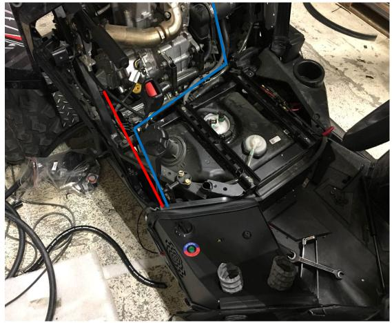
Connect heater switches with the heater harness.
