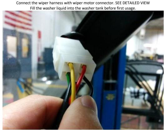
Connect the wiper/washer harness to the original electroinstallation.
