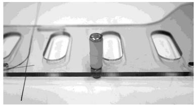
Now insert the bolt in the small holes and screw on the lock nuts so the end of the bolt is flush with the outside edge of the lock nut. Make sure that you place the bolt through hole on each slider so that they are mirror images of each other.
