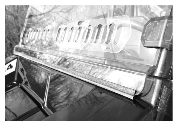
7. Then take the six Velcro clamps and place them through the square holes then wrap the strap around the roll cage and under the wire as shown in the photo below.
