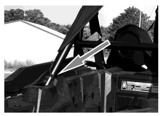
11. Finally make sure the top is centered and pull the straps tight. You may have to cut the ends of the straps and if you do make sure to melt the ends to prevent them from fraying out.
