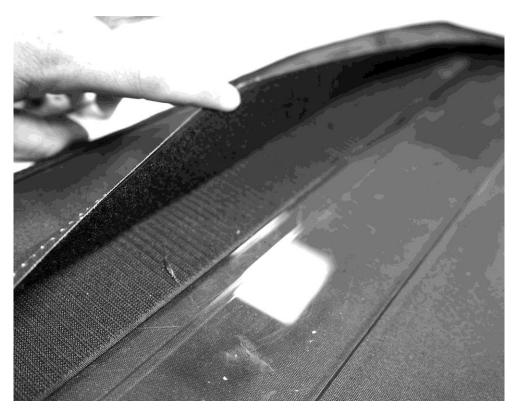
7. Now you are ready to install to front section on the RZR. Set it up on the plastic visor and fold the soft top back so the holes of the polycarbonate panel are exposed. Now take the two bolts you removed from the visor earlier and reinstall them through the panel and
