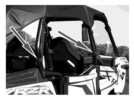
10. The last two straps attach to the end of the rear bars. Run the loop through the triangle hole where the two bars connect. See photo below
