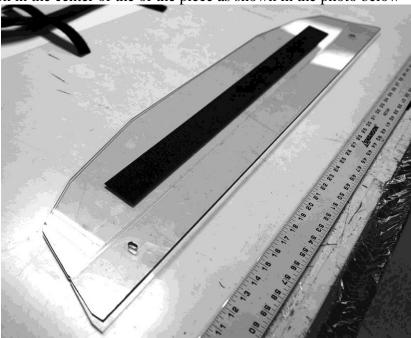
5. Next insert the polycarbonate panel into the pocket on the front of the soft top. Set it in the pocket as shown in the photo below making sure that the Velcro on the panel will match up with the Velcro sewn to the top.
