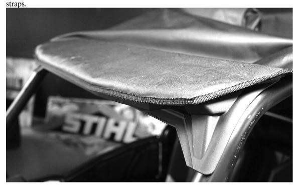
9. Now work your way around the rear of the vehicle and install the straps to tighten down the top. Wrap the looped end of the strap around the bars under the seat belt mount in the middle and under the cross bar on the second bar as shown in the photo below.
