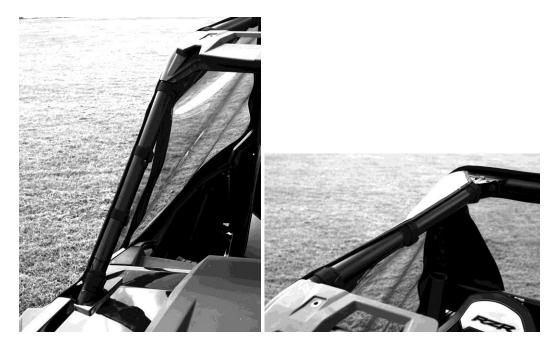
b. After installing the double-sided strips move to the rear of the door and attach the two Velcro tabs to the rear bar using the corresponding adhesive Velcro strip. See Photo Below:
