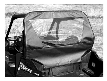
6. Prior to installing the top you must first remove the two front bolts that attach the front plastic piece to the frame. There are two bolts on each side but only remove the top bolt as shown in the photo below.
