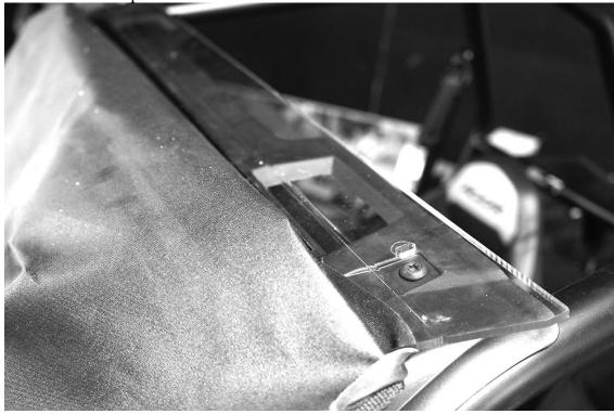
11. Now pull the soft top back over towards the rear of the vehicle and begin to install the six straps.
