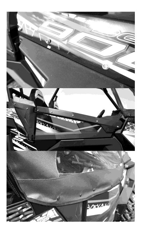
4. Installation of your Soft Rear Window is quite simple. Use the 24" strip and 5" strips to attach the rear window to the frame. It will also attach to the two double-sided tabs from the doors. Take the Soft Rear Window and attach it to the vehicle.
