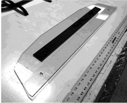
8. Next insert the polycarbonate panel into the pocket on the front of the soft top. Set it in the pocket as shown in the photo below making sure that the Velcro on the panel will match up with the Velcro sewn to the top.
