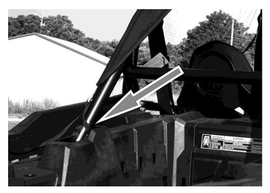
14. Finally make sure the top is centered and pull the straps tight. You may have to cut the ends of the straps and if you do make sure to melt the ends to prevent them from fraying out.
