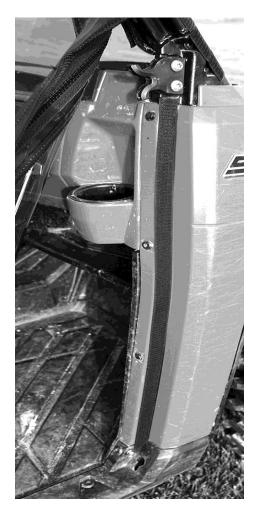
11. After all the Velcro is in place take the door and place it on the vehicle. the following series of photos show how it should look after being installed.
