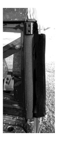
10. Now move to the front bottom edge of the door frame and install the 30" adhesive 1" wide Velcro strip. As shown in the photos on the next page.
