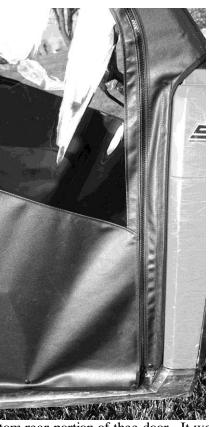
12. Lastly install the snap studs into the plastic for the bottom rear portion of thee door. It works best to put the screw studs into the snap sockets on the door first. Then one by one pull the door in place and push the screw into the plastic making sure to put enough pressure to leave a mark. Then remove the screw stud from the door and install it where the mark was left behind at. The following pictures show what it looks like.
