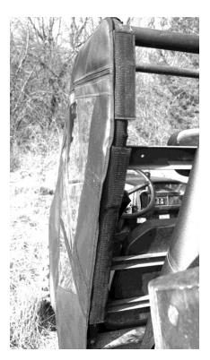
5. Once all the Velcro is in place the last thing to do is install the screw snap studs. NOTE: The best way to install the snap studs is to put them in the sockets in the door first. Then push them into the plastic to make a mark. Then pull the screw stud out and screw it into the plastic where the mark was made. See Photos Below.
