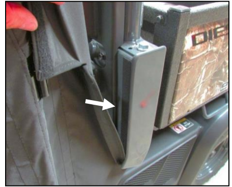
4. Adhere Velcro strips to rear flat part of the vehicle near the bed as shown. They should line up with Velcro on the fabric.
