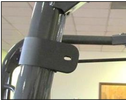
1. Place a clamp on the front roll cage bar. Refer to the picture below for locations.
