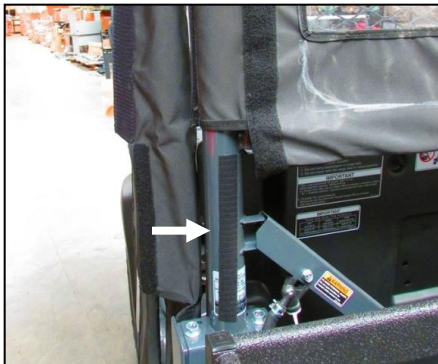
5. Adhere Velcro strips to the rear roll cage in the position shown. They should line up with the Velcro on the fabric.
