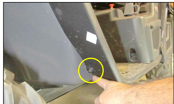
3. Place a clamp in the bottom rear corner of the roll cage in the location shown.
