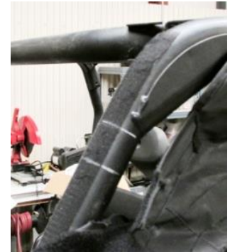
2. Mark position of light bar clamps on roll cage.
