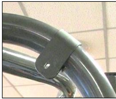
2. Place a clamp on the upper rear corner of the roll cage as shown above.
