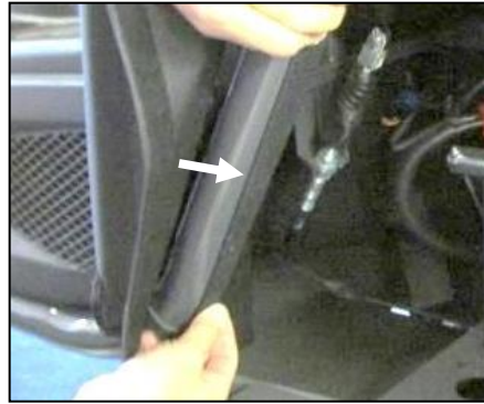
3. Adhere Velcro strap to the roll cage in the position shown above. They should line up with the Velcro on the subframe fabric.
