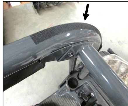
6. Adhere Velcro straps to upper front corner the roll cage as shown. They should line up with the Velcro on the fabric.
