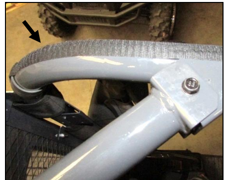
7. Adhere Velcro straps to upper rear corner the roll cage as shown. They should line up with the Velcro on the fabric.
