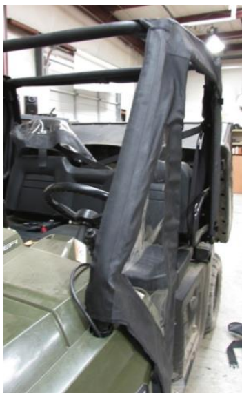
3. Remove bar & Install side panels to the front roll cage bars correctly.
