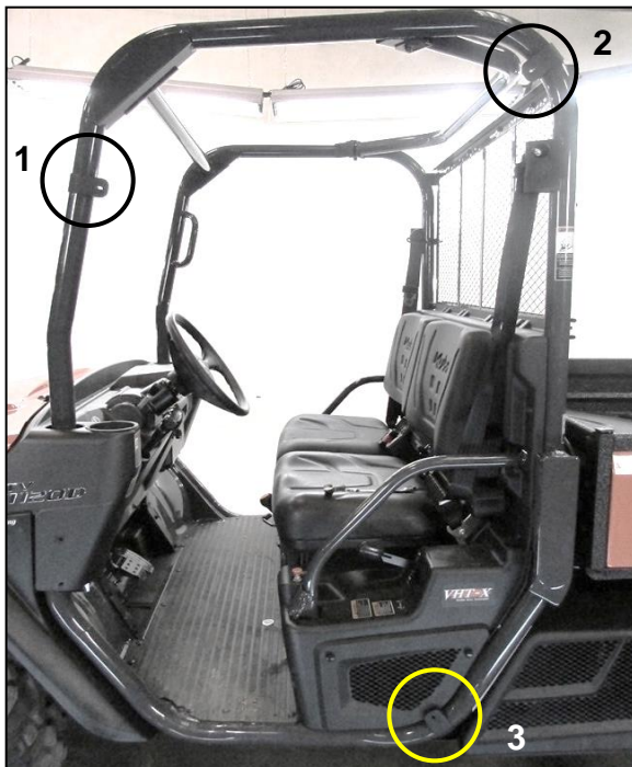
4. There should be 3 Plastic clamps in the locations shown.
