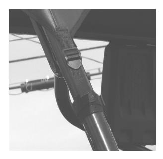
4. Then install the rear straps with the loop on the end. Run the strap around the end of the brace behind the seat and through the loop in the end of the strap. See Photo Below
