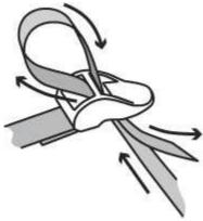
6. Once all four straps are in the buckles, pull them tight making sure to center the top and that the front edge of the top is an inch or so below the holes across the top of the windshield. Once the straps are pulled tight they should look like the picture below.
