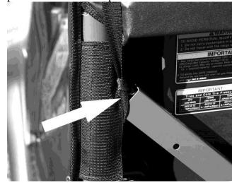
5. Now throw the Top Cap over the cab and attach it using the straps. Run the straps through the ladder lock buckles as shown in the diagram below.
